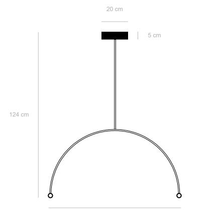
Materials: brass pipe, acrylic tube, LED lights Light: flexible LED strip light, 32W, 24V - UL listed
