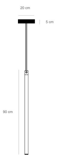
Materials: brass pipe, acrylic tube, LED lights Light: flexible LED strip light, 16W, 24V - UL listed
